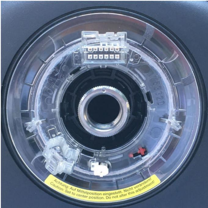
The OEM harness is made by 12 wires gathered in a 6 + 6 pin connector. The provided wire extension is made by a 6+6 pin harness. The connectors are not the same with the secure click-lock, but the pins need a bit of force to match the contacts, and they're not going to disconnect unless you apply a force which is much more than any dynamic action which may happen during driving.
