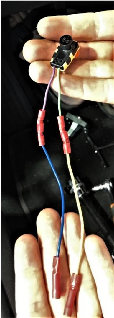
Go ahead crimping the 2 terminals to the wires coming out from the clockspring assembly. BE CAREFULL NOT TO MISMATCH THE WIRE COLORS. If a wire comes out from the clockspring , for example, in green, then the terminal must be crimped to the green wire that goes to the little airbag connector, and so the other one. Some cars does have 2 airbag connectors because of being dual stage airbag. In this case, repeat the procedure on the other connector.
