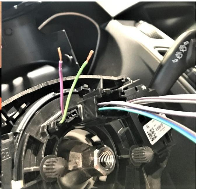
3) Purchase some wire, same AWG of your airbag wires, and cut 2 pieces, same length as the spacer, 5 to 6 cm (2" to 2" ½). Much better if the wires are the same color of your airbag wires. Peel the end of the wires as you did for the car's wires. Crimp 4 x terminals crimp-pipes fittings. You now made your extensions.
